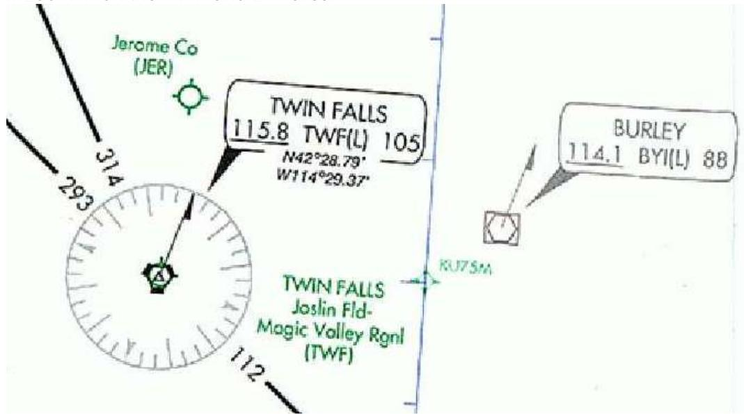
One thing we notice is that both VORs have a (L) after their VOR name. This means they are low altitude VORs, and in Flight Sim 2004, that means a 60 NM range. We'll go to the flight sim planner and figure out the mileage and heading information from TWF to BYI.
